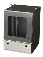
Saginaw workstation, NEMA 4/4X/12/13, 34 x 24 x 24in (HxWxD), desktop or pedestal mount, dual access, 304 stainless steel, #4 brush finish, single-door with keyboard drawer, 3-point keylocking flush swing handle, polycarbonate window.
