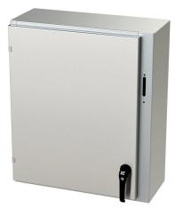
Saginaw Enviroline series disconnect enclosure, NEMA 3R/4/4X/12/13, right flange, 30 x 25 x 10in (HxWxD), wall mount, 304 stainless steel, #4 brush finish, single-door, 2-point padlocking handle, purchase subpanel separately.
