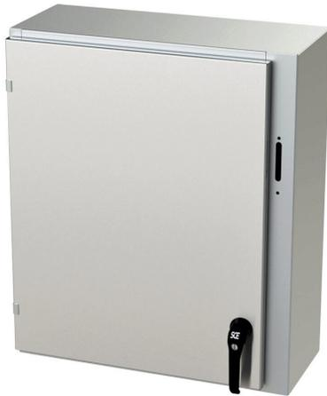
Saginaw Enviroline series disconnect enclosure, NEMA 3R/4/4X/12/13, right flange, 30 x 25 x 10in (HxWxD), wall mount, 316L stainless steel, #4 brush finish, single-door, 2-point padlocking handle, purchase subpanel separately.
