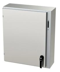
Saginaw Enviroline series disconnect enclosure, NEMA 3R/4/4X/12/13, right flange, 30 x 25 x 8in (HxWxD), wall mount, 304 stainless steel, #4 brush finish, single-door, 2-point padlocking handle, purchase subpanel separately.
