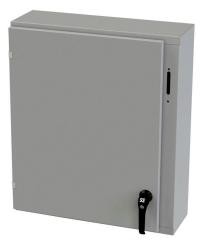
Saginaw Enviroline series disconnect enclosure, NEMA 3R/4/12/13, right flange, 30 x 25 x 8in (HxWxD), wall mount, carbon steel, ANSI 61 gray, powder coat finish, single-door, 2-point padlocking handle, purchase subpanel separately.
