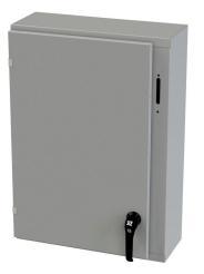
Saginaw Enviroline series disconnect enclosure, NEMA 3R/4/12/13, right flange, 30 x 21 x 8in (HxWxD), wall mount, carbon steel, ANSI 61 gray, powder coat finish, single-door, 2-point padlocking handle, purchase subpanel separately.
