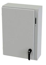
Saginaw Enviroline series disconnect enclosure, NEMA 3R/4/12/13, right flange, 30 x 21 x 8in (HxWxD), wall mount, carbon steel, RAL 7035 light gray, powder coat finish, single-door, 2-point padlocking handle, purchase subpanel separately.
