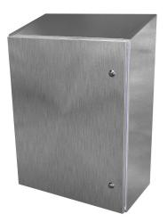
Saginaw sanitary enclosure, slope top, NEMA 3R/4/4X/12,  $30 \times 24 \times 12$ in (HxWxD), wall mount, 304 stainless steel, #4 brush finish, single-door, 1/4-turn sanitary stainless steel latch.
