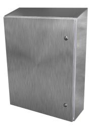
Saginaw sanitary enclosure, slope top, NEMA 3R/4/4X/12, 30 x 24 x 8in (HxWxD), wall mount, 304 stainless steel, #4 brush finish, single-door, 1/4-turn sanitary stainless steel latch.
