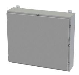
Saginaw enclosure, NEMA 3R/4/12/13, 30 x 36 x 8in (HxWxD), wall mount, carbon steel, ANSI 61 gray, powder coat finish, single-door, plated steel clamps, padlock hasp and staple.
