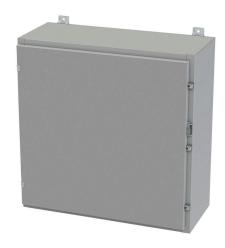
Saginaw enclosure, NEMA 3R/4/12/13, 30 x 30 x 12in (HxWxD), wall mount, carbon steel, ANSI 61 gray, powder coat finish, single-door, plated steel clamps, padlock hasp and staple.
