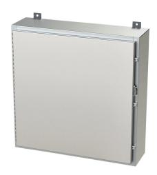
Saginaw enclosure, NEMA 3R/4/4X/12/13, 30 x 30 x 8in (HxWxD), wall mount, 304 stainless steel, #4 brush finish, single-door, stainless steel clamps, padlock hasp and staple.
