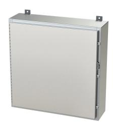
Saginaw enclosure, NEMA 3R/4/4X/12/13, 30 x 30 x 8in (HxWxD), wall mount, 316L stainless steel, #4 brush finish, single-door, stainless steel clamps, padlock hasp and staple.
