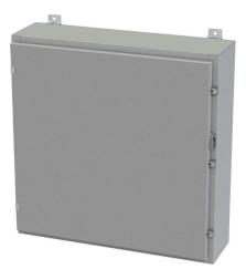
Saginaw enclosure, NEMA 3R/4/12/13, 30 x 30 x 8in (HxWxD), wall mount, carbon steel, ANSI 61 gray, powder coat finish, single-door, plated steel clamps, padlock hasp and staple.
