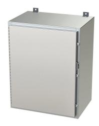
Saginaw enclosure, NEMA 3R/4/4X/12/13, 30 x 24 x 16in (HxWxD), wall mount, 304 stainless steel, #4 brush finish, single-door, stainless steel clamps, padlock hasp and staple.
