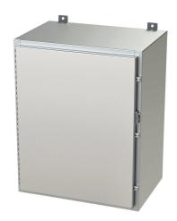
Saginaw enclosure, NEMA 3R/4/4X/12/13, 30 x 24 x 16in (HxWxD), wall mount, 316L stainless steel, #4 brush finish, single-door, stainless steel clamps, padlock hasp and staple.
