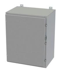
Saginaw enclosure, NEMA 3R/4/12/13, 30 x 24 x 16in (HxWxD), wall mount, carbon steel, ANSI 61 gray, powder coat finish, single-door, plated steel clamps, padlock hasp and staple.
