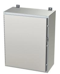
Saginaw enclosure, NEMA 3R/4/4X/12/13, 30 x 24 x 12in (HxWxD), wall mount, 304 stainless steel, #4 brush finish, single-door, stainless steel clamps, padlock hasp and staple.
