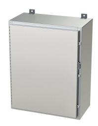
Saginaw enclosure, NEMA 3R/4/4X/12/13, 30 x 24 x 12in (HxWxD), wall mount, 316L stainless steel, #4 brush finish, single-door, stainless steel clamps, padlock hasp and staple.
