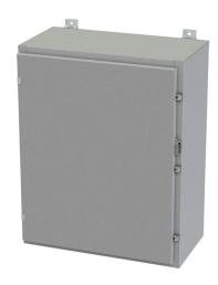
Saginaw enclosure, NEMA 3R/4/12/13, 30 x 24 x 12in (HxWxD), wall mount, carbon steel, ANSI 61 gray, powder coat finish, single-door, plated steel clamps, padlock hasp and staple.
