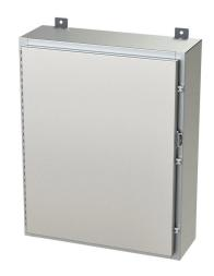
Saginaw enclosure, NEMA 3R/4/4X/12/13, 30 x 24 x 8in (HxWxD), wall mount, 304 stainless steel, #4 brush finish, single-door, stainless steel clamps, padlock hasp and staple.
