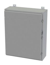
Saginaw enclosure, NEMA 3R/4/12/13, 30 x 24 x 8in (HxWxD), wall mount, carbon steel, ANSI 61 gray, powder coat finish, single-door, plated steel clamps, padlock hasp and staple.
