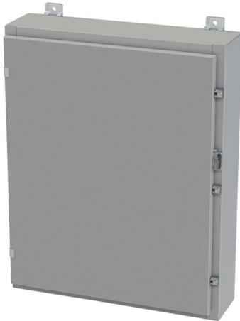
Saginaw enclosure, NEMA 3R/4/12/13, 30 x 24 x 6in (HxWxD), wall mount, carbon steel, ANSI 61 gray, powder coat finish, single-door, plated steel clamps, padlock hasp and staple.
