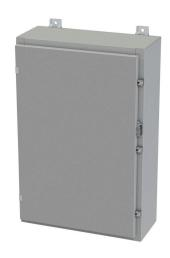
Saginaw enclosure, NEMA 3R/4/12/13, 30 x 20 x 8in (HxWxD), wall mount, carbon steel, ANSI 61 gray, powder coat finish, single-door, plated steel clamps, padlock hasp and staple.
