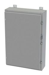
Saginaw enclosure, NEMA 3R/4/12/13, 30 x 20 x 6in (HxWxD), wall mount, carbon steel, ANSI 61 gray, powder coat finish, single-door, plated steel clamps, padlock hasp and staple.
