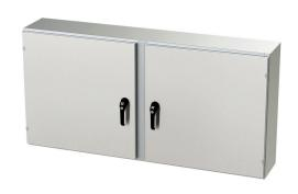
Saginaw Enviroline series enclosure, NEMA 3R/4/4X/12/13, 30 x 60 x 10in (HxWxD), wall mount, 304 stainless steel, #4 brush finish, 2-door, 3-point keylocking/padlocking combo handle.
