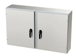
Saginaw Enviroline series enclosure, NEMA 3R/4/4X/12/13, 30 x 48 x 10in (HxWxD), wall mount, 304 stainless steel, #4 brush finish, 2-door, 3-point keylocking/padlocking combo handle.
