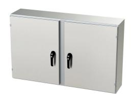
Saginaw Enviroline series enclosure, NEMA 3R/4/4X/12/13,  $30 \times 48 \times 10$ in (HxWxD), wall mount, 304 stainless steel, #4 brush finish, 2-door, 3-point keylocking/padlocking combo handle.
