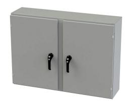
Saginaw Enviroline series enclosure, NEMA 3R/4/12/13, 30 x 42 x 10in (HxWxD), wall mount, carbon steel, ANSI 61 gray, powder coat finish, 2-door, 3-point keylocking/padlocking combo handle.
