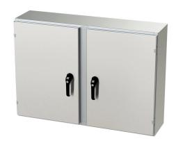
Saginaw Enviroline series enclosure, NEMA 3R/4/4X/12/13,  $30 \times 42 \times 10$ in (HxWxD), wall mount, 304 stainless steel, #4 brush finish, 2-door, 3-point keylocking/padlocking combo handle.
