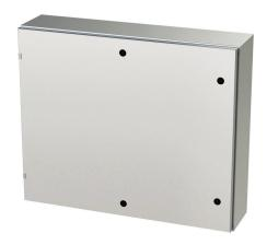
Saginaw Enviroline series enclosure, NEMA 3R/4/4X/12/13, 30 x 36 x 8in (HxWxD), wall mount, 304 stainless steel, #4 brush finish, single-door, 1/4-turn semi-flush latch.
