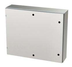
Saginaw Enviroline series enclosure, NEMA 3R/4/4X/12/13,  $30 \times 36 \times 8$  in (HxWxD), wall mount, 316L stainless steel, #4 brush finish, single-door, 1/4-turn semi-flush latch.
