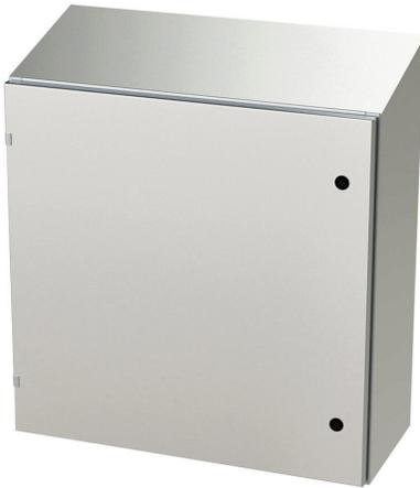
Saginaw Enviroline series enclosure, slope top, NEMA 3R/4/4X/12/13, 30 x 30 x 12in (HxWxD), wall mount, 304 stainless steel, #4 brush finish, single-door, 1/4-turn semi-flush latch.
