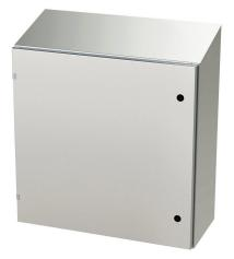
Saginaw Enviroline series enclosure, slope top, NEMA 3R/4/4X/12/13,  $30 \times 30 \times 12in$  (HxWxD), wall mount, 304 stainless steel, #4 brush finish, single-door, 1/4-turn semi-flush latch.
