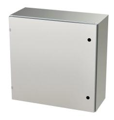
Saginaw Enviroline series enclosure, NEMA 3R/4/4X/12/13,  $30 \times 30 \times 12$ in (HxWxD), wall mount, 304 stainless steel, #4 brush finish, single-door, 1/4-turn semi-flush latch.
