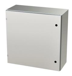
Saginaw Enviroline series enclosure, NEMA 3R/4/4X/12/13, 30 x 30 x 12in (HxWxD), wall mount, 316L stainless steel, #4 brush finish, single-door, 1/4-turn semi-flush latch.
