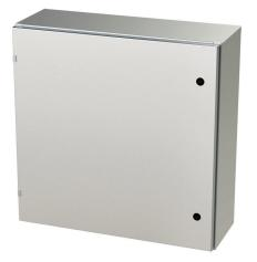
Saginaw Enviroline series enclosure, NEMA 3R/4/4X/12/13,  $30 \times 30 \times 10$ in (HxWxD), wall mount, 316L stainless steel, #4 brush finish, single-door, 1/4-turn semi-flush latch.
