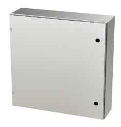
Saginaw Enviroline series enclosure, NEMA 3R/4/4X/12/13,  $30 \times 30 \times 8$  in (HxWxD), wall mount, 304 stainless steel, #4 brush finish, single-door, 1/4-turn semi-flush latch.
