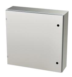
Saginaw Enviroline series enclosure, NEMA 3R/4/4X/12/13,  $30 \times 30 \times 8$  in (HxWxD), wall mount, 316L stainless steel, #4 brush finish, single-door, 1/4-turn semi-flush latch.
