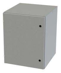
Saginaw Enviroline series enclosure, NEMA 3R/4/12/13, 30 x 24 x 24in (HxWxD), wall mount, carbon steel, ANSI 61 gray, powder coat finish, single-door, 1/4-turn semi-flush latch.
