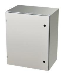
Saginaw Enviroline series enclosure, NEMA 3R/4/4X/12/13,  $30 \times 24 \times 16$  in (HxWxD), wall mount, 304 stainless steel, #4 brush finish, single-door, 1/4-turn semi-flush latch.
