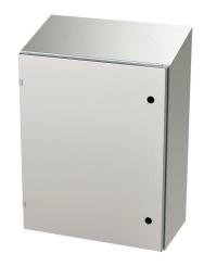
Saginaw Enviroline series enclosure, slope top, NEMA 3R/4/4X/12/13, 30 x 24 x 12in (HxWxD), wall mount, 304 stainless steel, #4 brush finish, single-door, 1/4-turn semi-flush latch.
