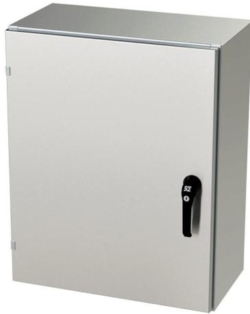
Saginaw Enviroline series enclosure, NEMA 3R/4/4X/12/13, 30 x 24 x 12in (HxWxD), wall mount, 304 stainless steel, #4 brush finish, single-door, 3-point keylocking/padlocking combo handle.
