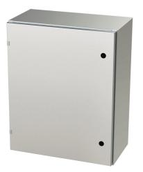
Saginaw Enviroline series enclosure, NEMA 3R/4/4X/12/13,  $30 \times 24 \times 12$ in (HxWxD), wall mount, 316L stainless steel, #4 brush finish, single-door, 1/4-turn semi-flush latch.
