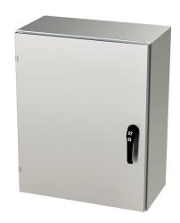
Saginaw Enviroline series enclosure, NEMA 3R/4/4X/12/13,  $30 \times 24 \times 12$ in (HxWxD), wall mount, 316L stainless steel, #4 brush finish, single-door, 3-point keylocking/padlocking combo handle.
