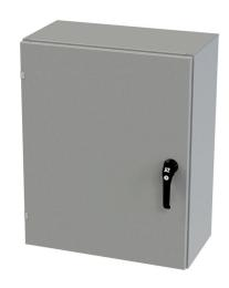
Saginaw Enviroline series enclosure, NEMA 3R/4/12/13, 30 x 24 x 12in (HxWxD), wall mount, carbon steel, ANSI 61 gray, powder coat finish, single-door, 3-point keylocking/padlocking combo handle.
