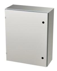
Saginaw Enviroline series enclosure, NEMA 3R/4/4X/12/13,  $30 \times 24 \times 10$  in (HxWxD), wall mount, 304 stainless steel, #4 brush finish, single-door, 1/4-turn semi-flush latch.
