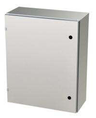
Saginaw Enviroline series enclosure, NEMA 3R/4/4X/12/13,  $30 \times 24 \times 10$ in (HxWxD), wall mount, 316L stainless steel, #4 brush finish, single-door, 1/4-turn semi-flush latch.
