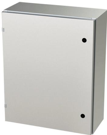
Saginaw Enviroline series enclosure, NEMA 3R/4/4X/12/13, 30 x 24 x 10in (HxWxD), wall mount, 316L stainless steel, #4 brush finish, single-door, 1/4-turn semi-flush latch.
