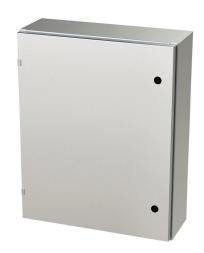
Saginaw Enviroline series enclosure, NEMA 3R/4/4X/12/13,  $30 \times 24 \times 8$  in (HxWxD), wall mount, 304 stainless steel, #4 brush finish, single-door, 1/4-turn semi-flush latch.
