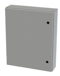
Saginaw Enviroline series enclosure, NEMA 3R/4/12/13,  $30 \times 24 \times 6$  in (HxWxD), wall mount, carbon steel, ANSI 61 gray, powder coat finish, single-door, 1/4-turn semi-flush latch.
