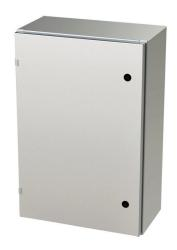
Saginaw Enviroline series enclosure, NEMA 3R/4/4X/12/13, 30 x 20 x 10in (HxWxD), wall mount, 316L stainless steel, #4 brush finish, single-door, 1/4-turn semi-flush latch.
