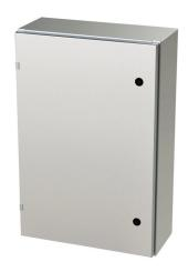
Saginaw Enviroline series enclosure, NEMA 3R/4/4X/12/13,  $30 \times 20 \times 8$  in (HxWxD), wall mount, 304 stainless steel, #4 brush finish, single-door, 1/4-turn semi-flush latch.
